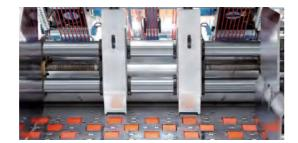
Leading-edge Feeder System Self-developed leading-edge feed system specially for deformed, warped corrugated papers.
