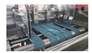
The unique belt feed specially applies for all kind of thick and thin cardboard paper, improve the lamination accuracy. Minimum bottom paper thickness is 300gsm.
