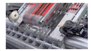
Paper Aligning System Full-servo tracking system to ensure stability and highprecision.
