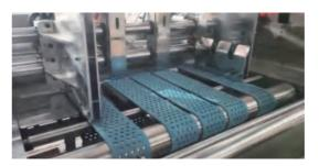
The unique belt feed specially applies for all kind of thick and thin cardboard paper, improve the lamination accuracy. Minimum bottom paper thickness is 300gsm.
