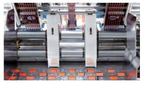
Leading-edge Feeder System Self-developed leading-edge feed system specially for deformed, warped corrugated papers.
