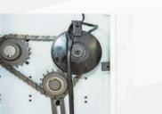
Sheet Delivery **Individual Control** Individual drive structure for AB sheet feeding to avoid the scratches.
